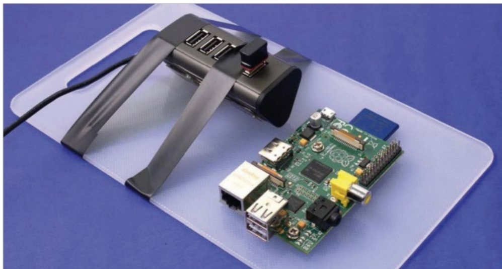
■ The Raspberry Pi with SD card and the powered USB hub fastened in position, ready to go into the folder
